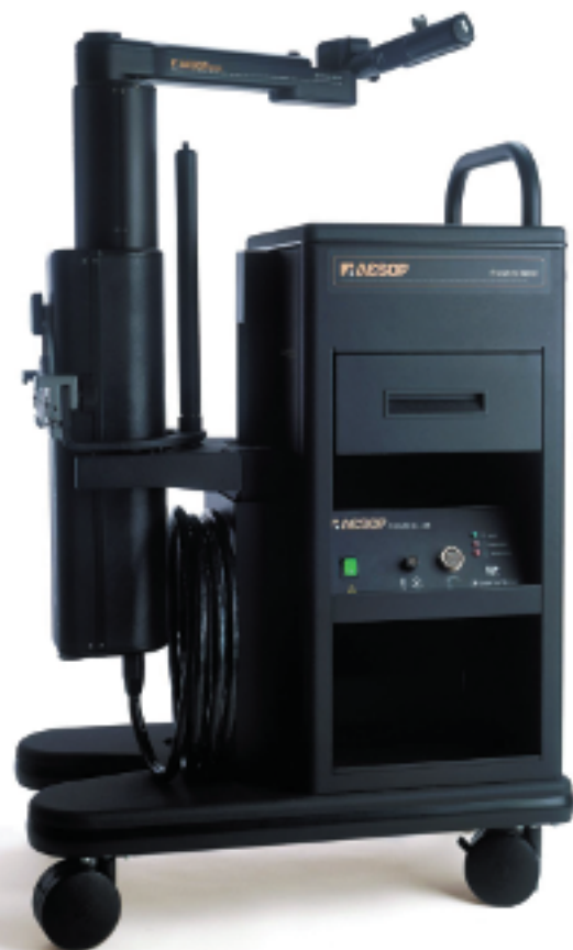
FIGURE 39-1. The AESOP 3000 robotic arm (Courtesy of Intuitive Surgical, Sunnyvale, CA; with permission).
